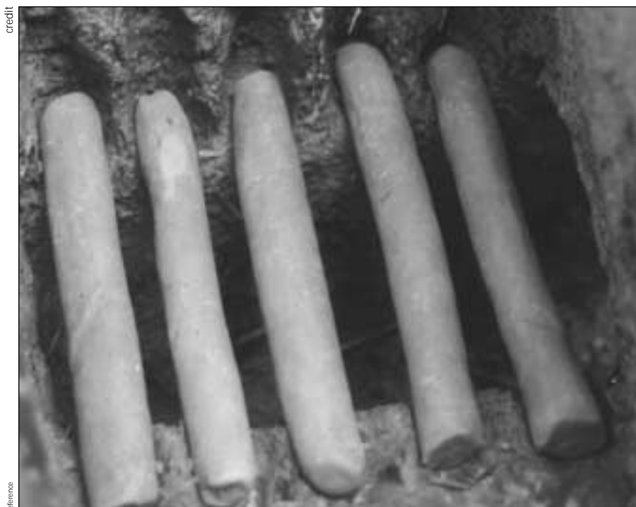
Figure 5: Rods in position in a stove, forming the grate over the ash hole.
