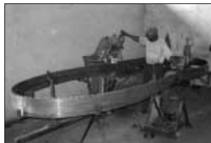
Figure 2: Sawdoctor sharpening saw blade in Forest Africana Sawmill, Kumasi, Ghana3
