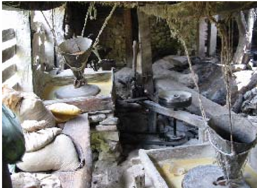
Fig. 6 Upgraded Ghatta with two grinders
