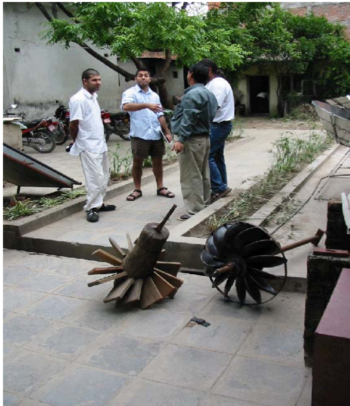
Fig. 5 Old and New Ghatta Turbines
