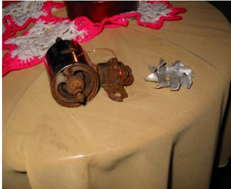
Fig. 13 This 200 IRs ($4 US) Pico Hydro Generator operated 24 hours a day for more than two years
