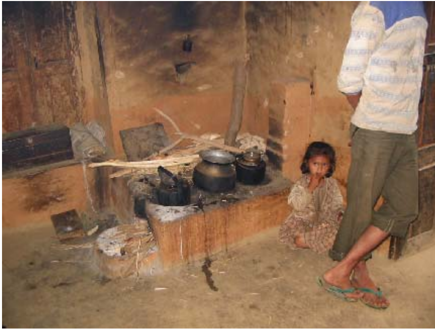
Fig. 9 150 NRs ($2 US) Clay stove with chimney, Nepal
